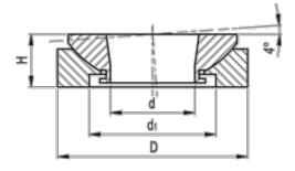
$\begin{array}{lll} D & = 45 \\ d & = 20 \\ d1 & = 30 \\ H & = 12.5 \\ Max \ screw \ dimension = M16 \\ Static \ load \ (kN) & = 120 \\ Weight \ (g) & = 104 \\ \end{array}$
